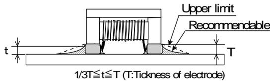
Accordingly increasing the solder volume, the mechanical stress to Chip is also increased. Exceeding solder volume may cause the failure of mechanical or electrical performance.
