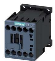
Coupling contactor relay, 3 NO + 1 NC, 110 V DC, 0.7 ... 1.25\* US, with integrated suppressor diode, Size S00, screw terminal suitable for PLC outputs
