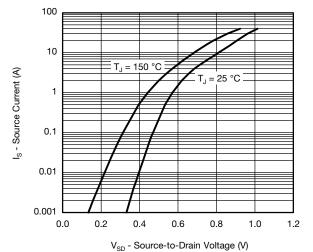
Source-Drain Diode Forward Voltage
