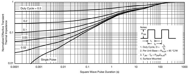
Normalized Thermal Transient Impedance, Junction-to-Ambient
