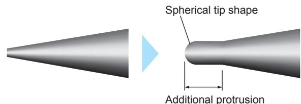
The discharge needle tip's spherical shape enables more stable ion production while making it less likely that the shape of the tip will change over time as a result of electrical discharge.
