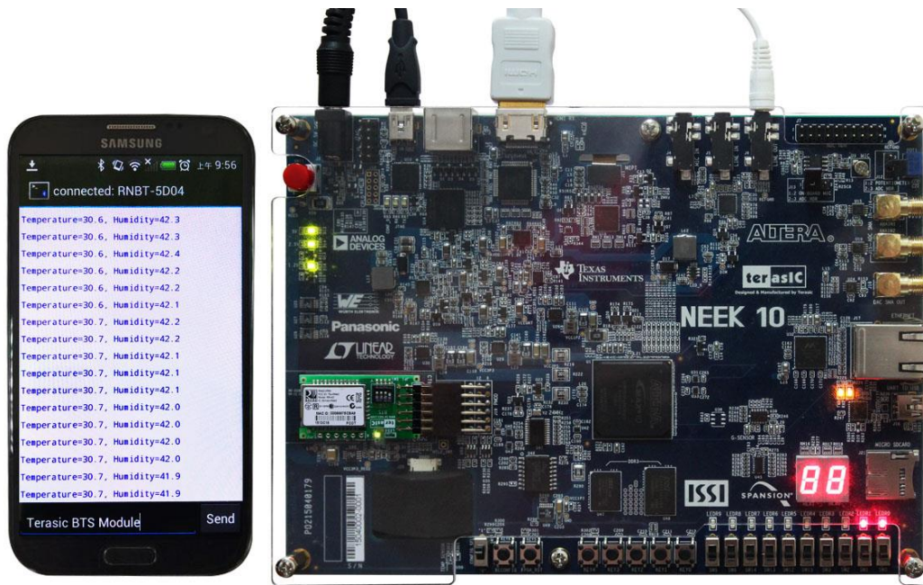
Figure 4-5 The data gathered on a smartphone after executing the demonstration
