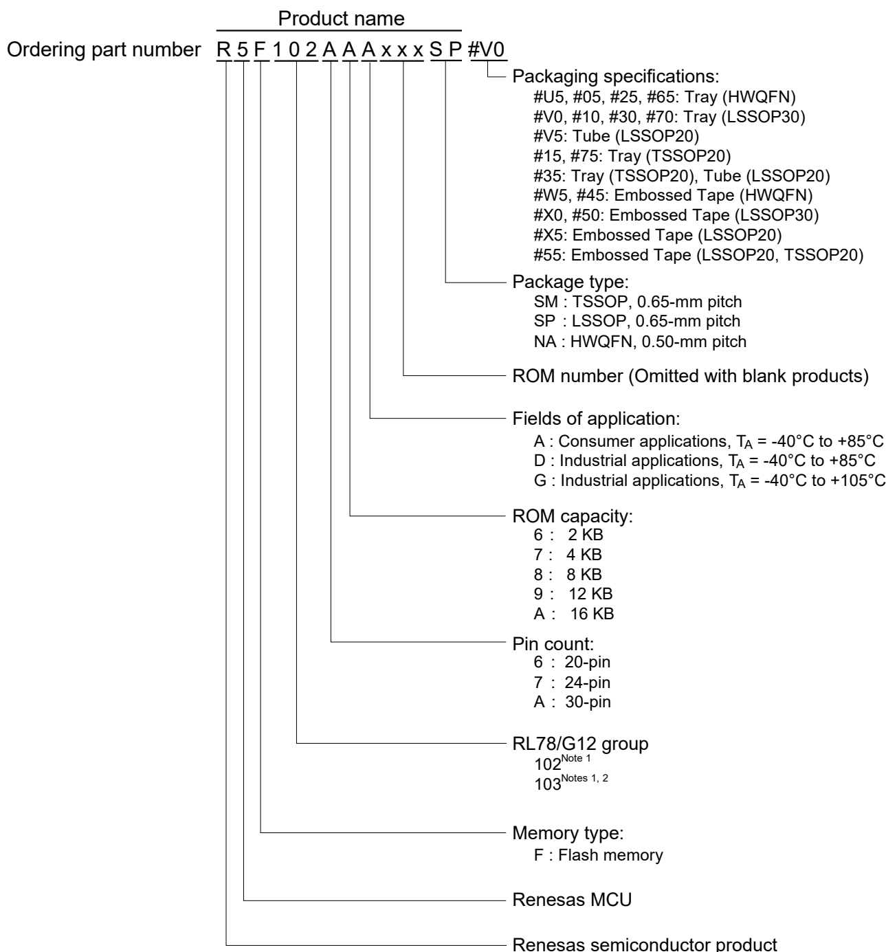
Figure 1-1. Part Number, Memory Size, and Package of RL78/G12
