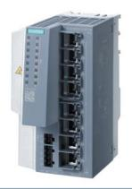
SCALANCE XCM108PoE (8x100 Mbit/s RJ45, PoE) unmanaged IE Switch up to 120 W PoE power on 8 ports, LED diagnostics, error-signaling contact with set pushbutton, redundant power supply manual available as a download .
