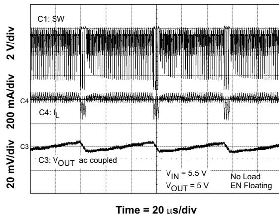
Figure 21. Low Dropout Operation
