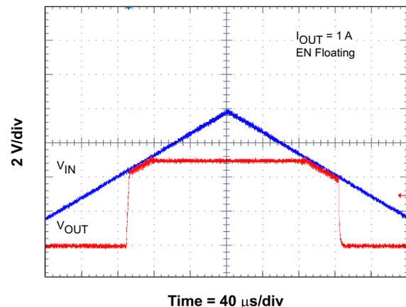
Figure 22. Low Dropout Start Up and Shutdown
