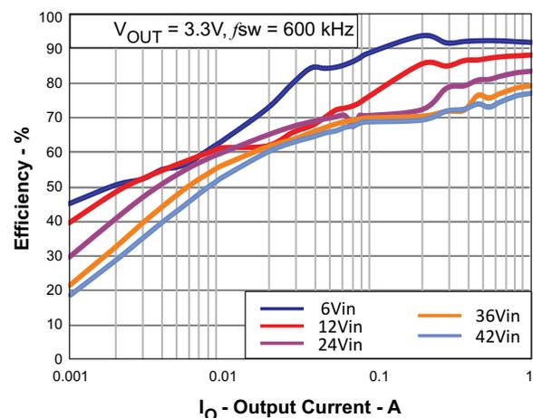
**Figure 3. Light-Load Efficiency**
