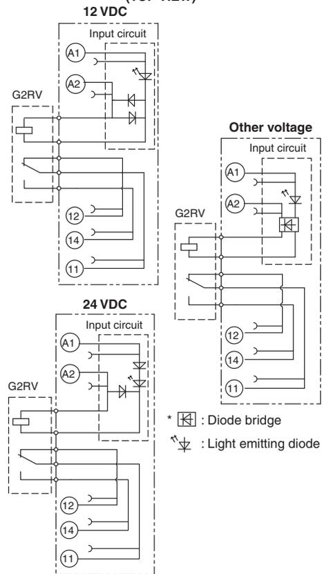
**Models with latching lever (with test switch)**
