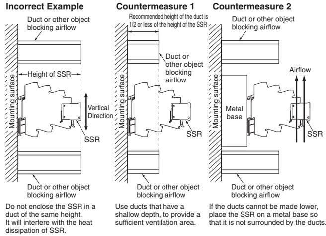
Do not enclose the SSR in a duct of the same height. It will interfere with the heat dissipation of SSR.
