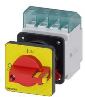
SENTRON, Switch disconnector 3LD, emergency switching-off switch, 4- pole, lu: 16 A, operating power / at AC-23 A 400 V: 7.5 kW, front-mounted, knob-operated mechanism, Red / yellow, central mounting 22.5 mm of the handle
