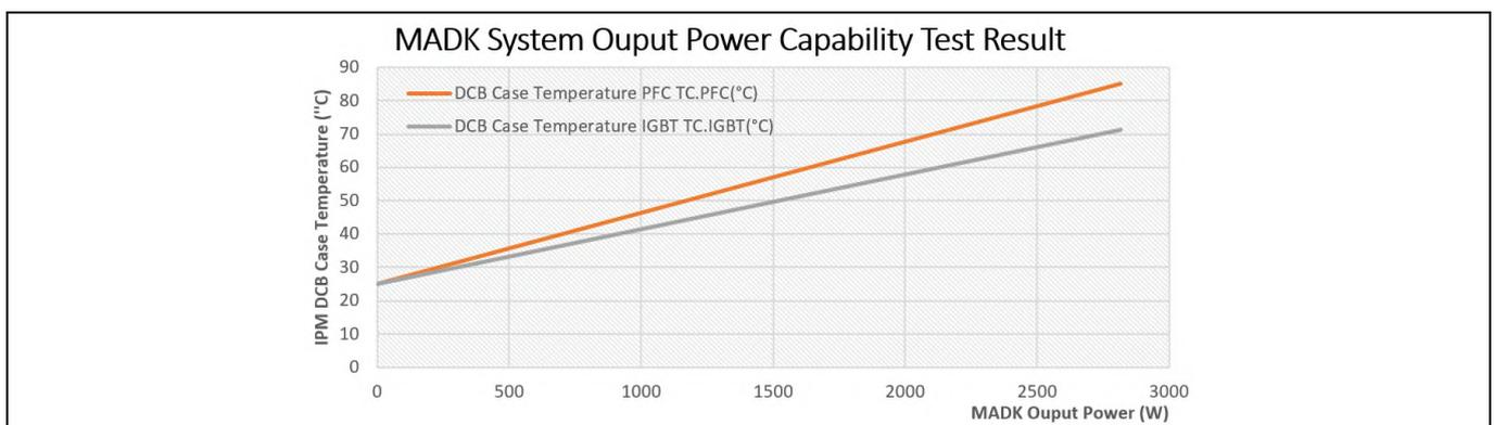
**Figure 31 MADK output power capability test result**
