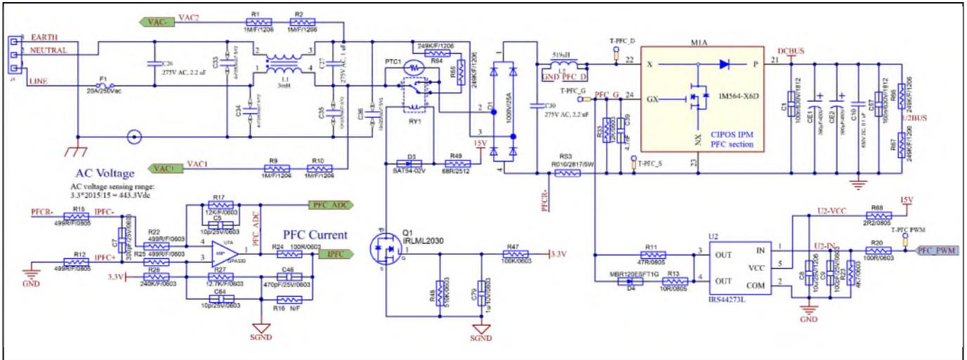
**Figure 33 PFC section schematics for EVAL-M3- IM564**
