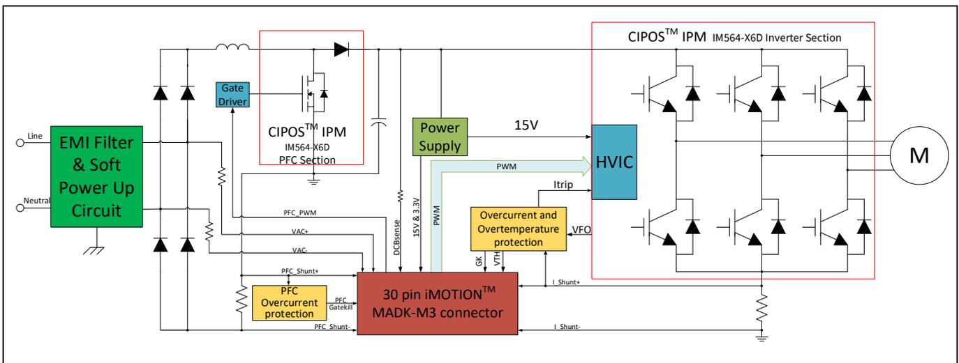
**Figure 1 The block diagram of the EVAL-M3-IM564**
