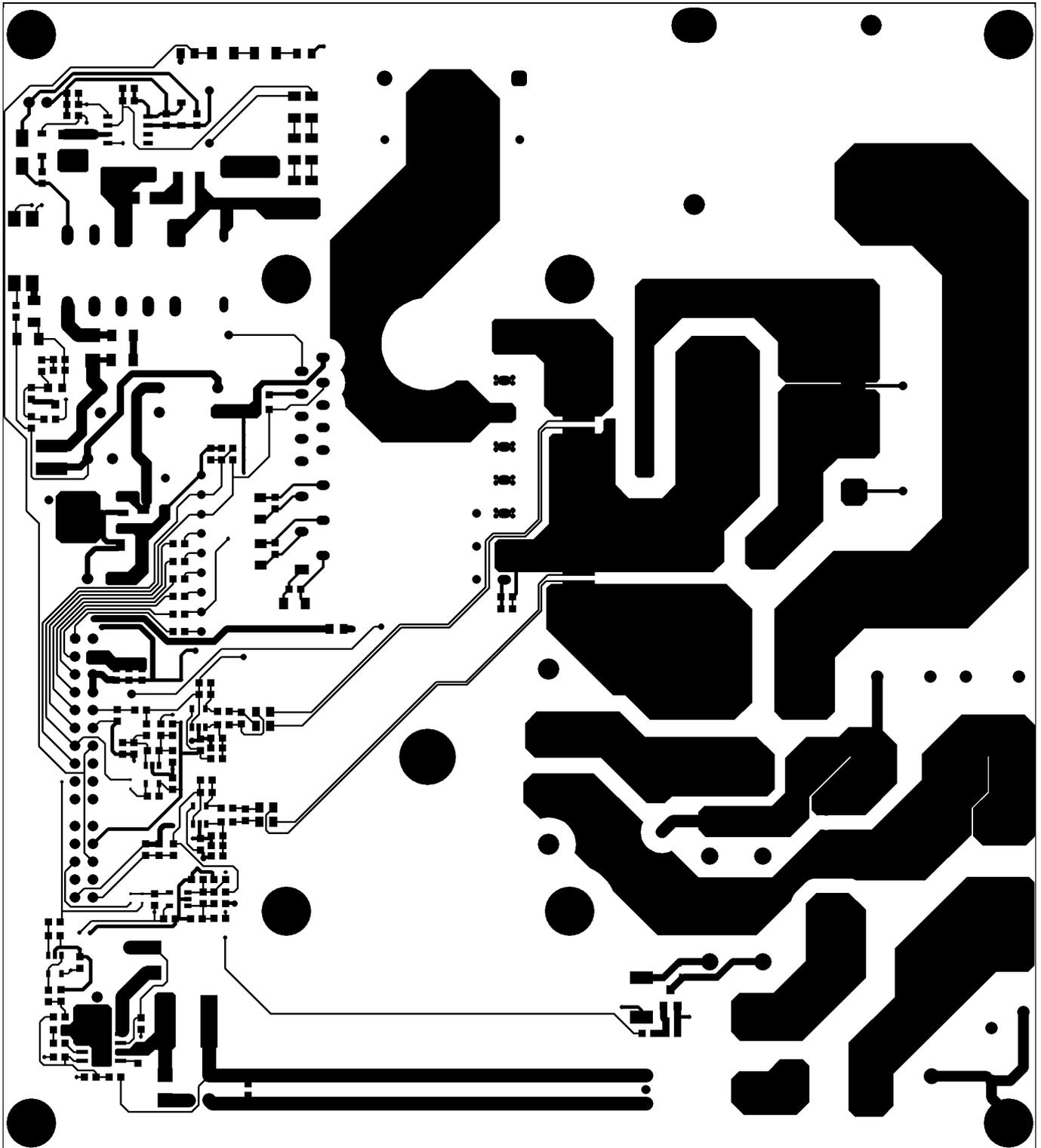
**Figure 38** Top layer routing of the EVAL-M3-IM564
