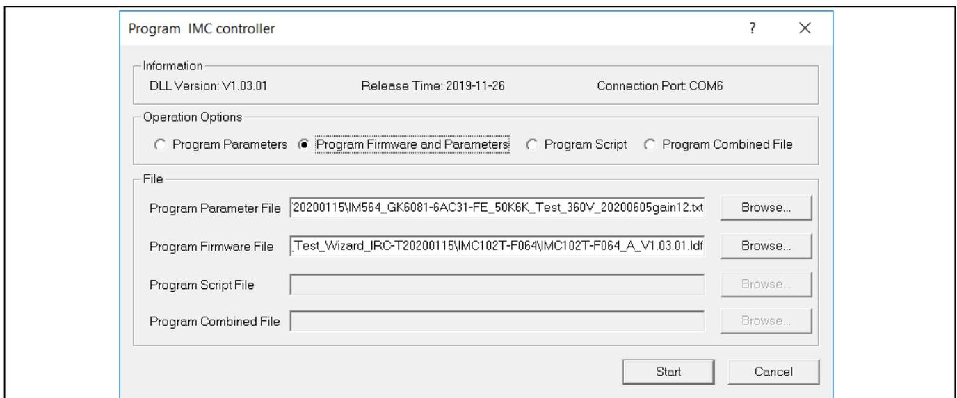
**Figure 9 Program firmware and parameter in “Program IMC Controller” pop-up window**
