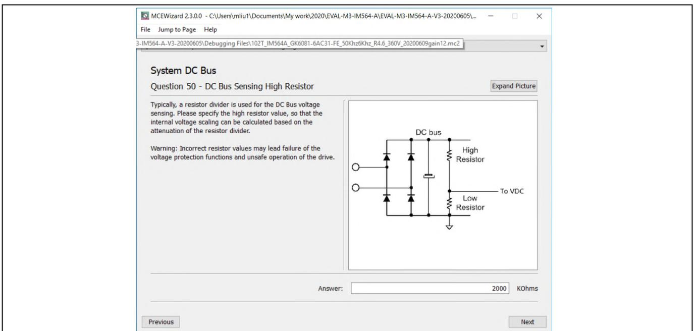
**Figure 20 DC bus sensing configuration in MCEWizard**
