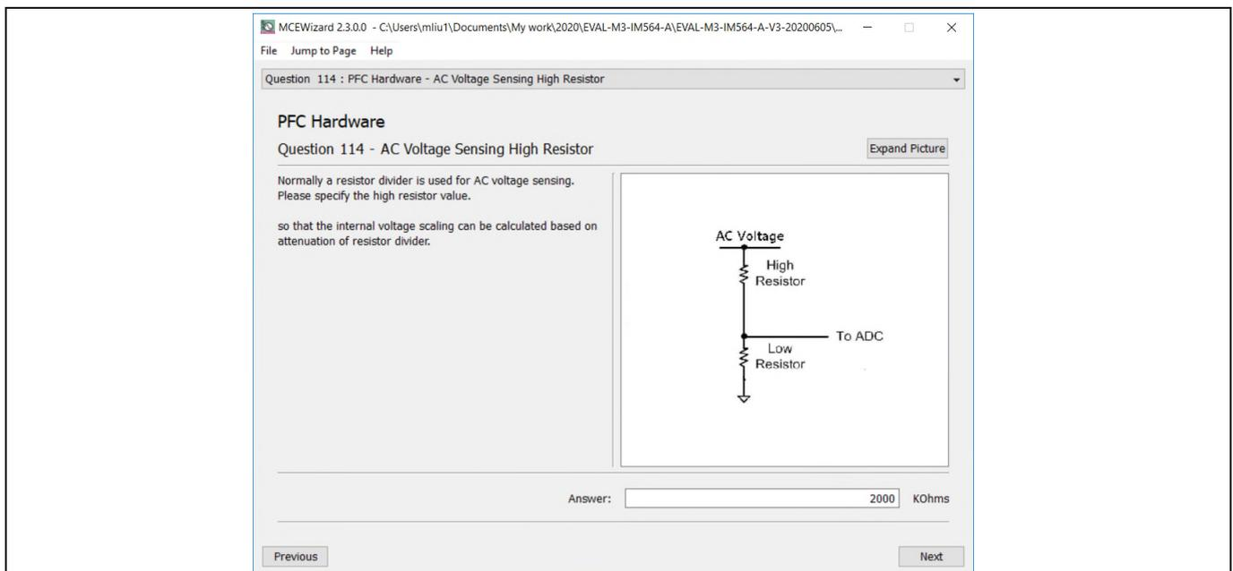
**Figure 13 AC voltage sensing configuration in MCEWizard**
