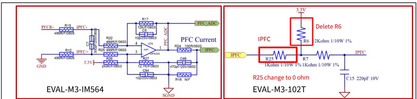
**Figure 15 The PFC current feedback circuit for EVAL-M3-102T evaluation board**
