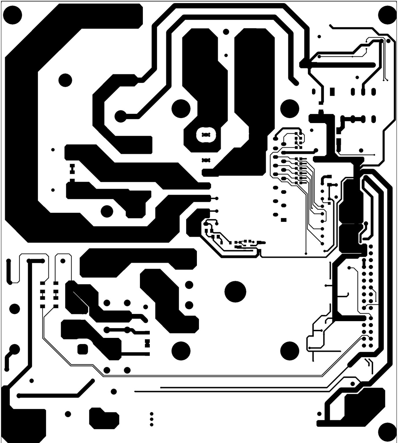
**Figure 39** Bottom layer routing of the EVAL-M3-IM564
