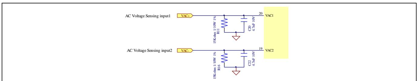
**Figure 11 The AC voltage sensing schematic of EVAL-M3-102T**
