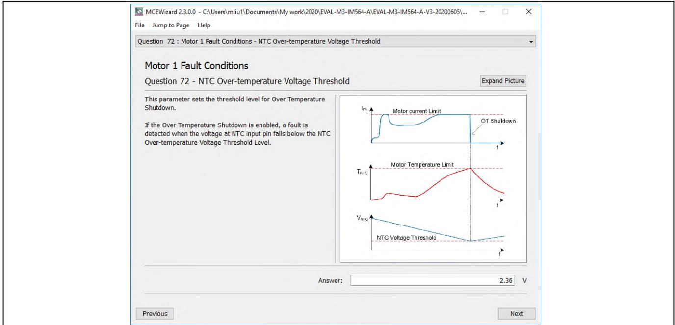
**Figure 28 External temperature sense input configuration in MCEWizard**
