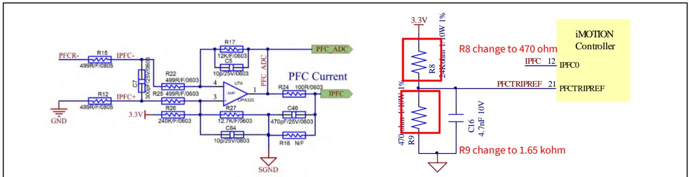
**Figure 16 PFC OCP1 on the EVAL-M3-IM564 evaluation board**
