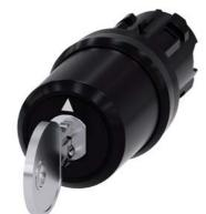
Key-operated switch BKS, 22 mm, round, plastic, lock number S1, with 2 keys, 3 switch positions I-O-II, latching, actuating angle 2x45°, 10:30h/12h/13:30h, key removal II
