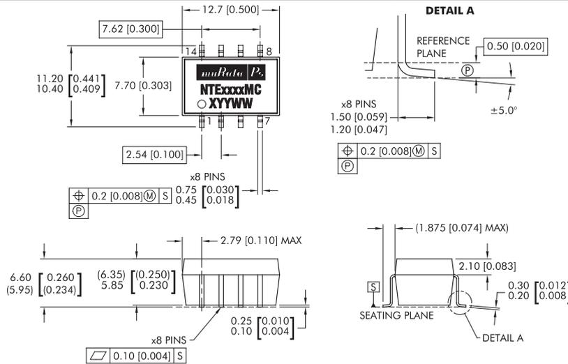
All dimensions in mm (inches), Controlling dimension is mm. Tolerances (unless otherwise stated) ±0.25 (0.010).
