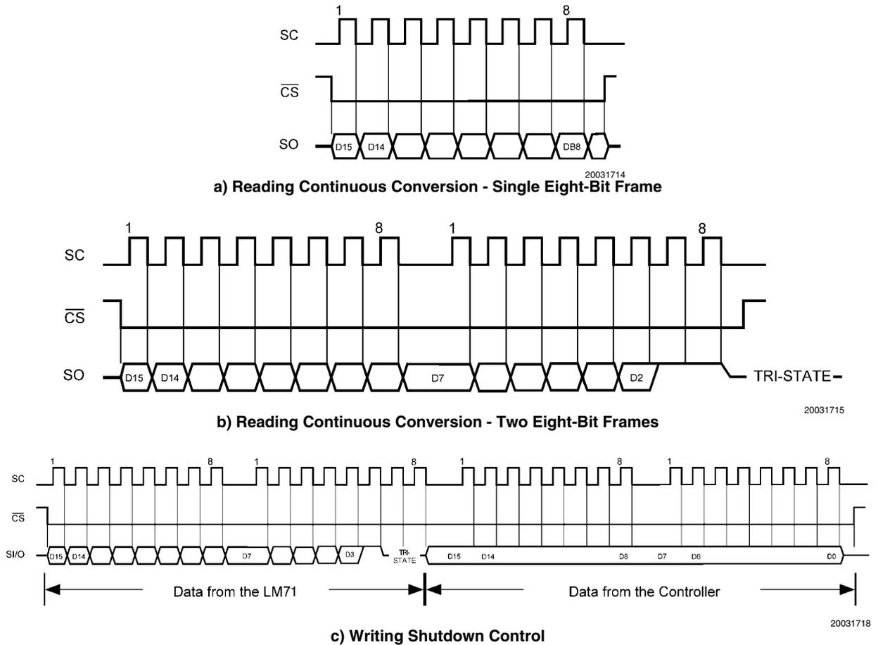
FIGURE 7. Timing Diagrams
