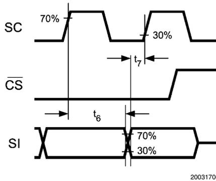
FIGURE 4. Data Input Timing Diagram
