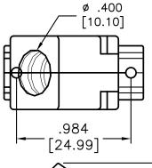
Connector Cover Material: ABS Compound Nickel Plated
