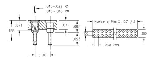
**Description:** Interconnect Socket .100 Grid; Straight Socket Ultra Low Profile Double Row Through Hole Accepts .015-.022" Leads Plating Code:
