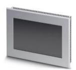
Touch panel with 17.8 cm/7" TFT-display (analog resistive (polyester)), 800 x 480 Pixel(s) (WVGA), 65536 colors, ARM9<sup>™</sup>, 200 MHz, 2x USB host 2.0, 1 x Ethernet (10/100 Mbps), RJ45, Windows CE 5.0 and user software: Open platform. (bus system: without)
