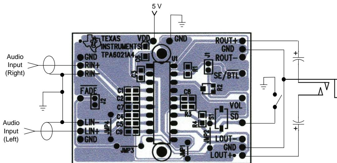
Figure 3. TPA6021A4 EVM Connected for Stereo Single-Ended Output
