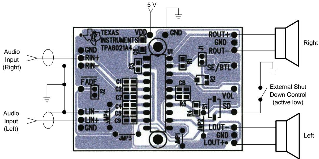
Figure 2. TPA6021A4 EVM Connected for Stereo BTL Output
