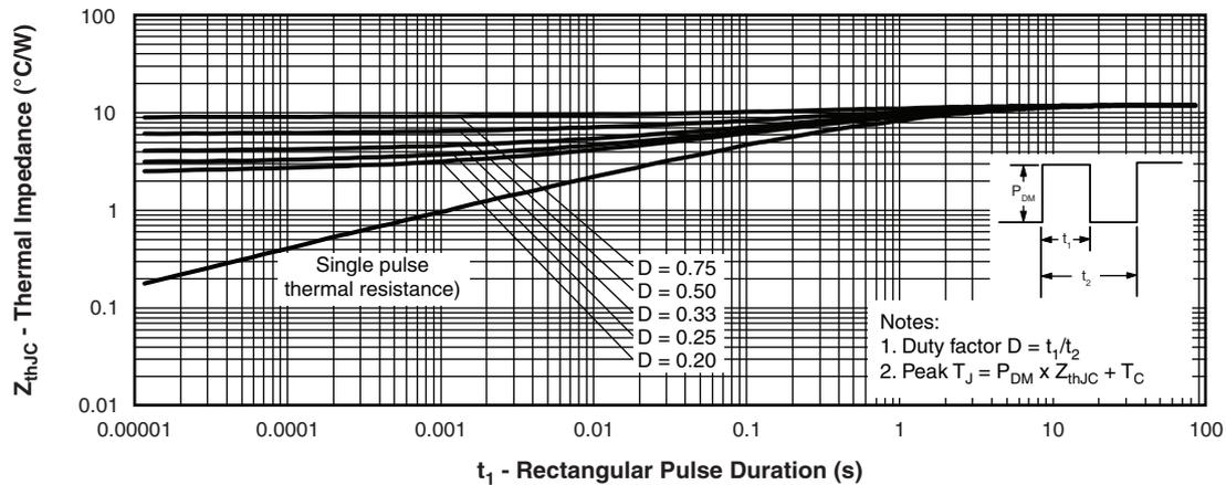
Fig. 4 - Maximum Thermal Impedance  $Z_{thJC}$  Characteristics (Per Leg)
