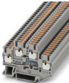
Component terminal block, connection method: Push-in connection, cross section: 0.14 mm 2 - 4 mm 2 , AWG: 26 - 12, width: 5.2 mm, color: gray, mounting type: NS 35/7,5, NS 35/15
