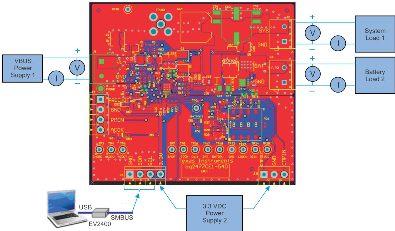
**Figure 3. Original Test Setup for PWR540 (bq2477xEVM)**
