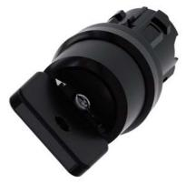
Key-operated switch O.M.R, 22 mm, round, plastic, lock number 73034, black, with 2 keys, 2 switch positions O-I, latching, actuating angle 90°, 10:30h/13:30h, Key removal I
