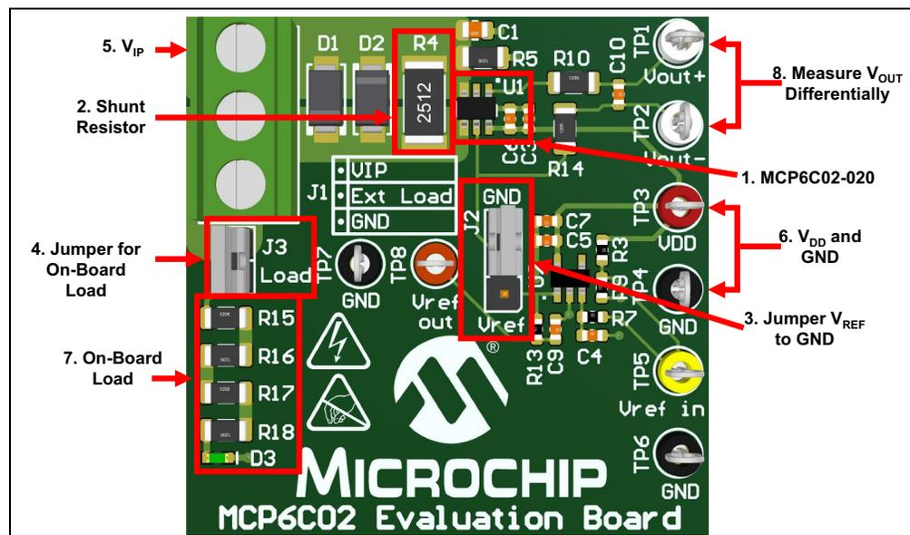
**FIGURE 2-3:** Out-of-the-Box Setup.
