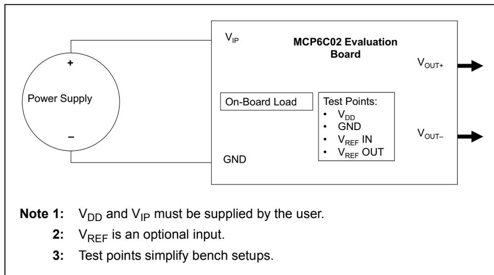
**FIGURE 1-2:** Using the On-Board Load Block Diagram.
