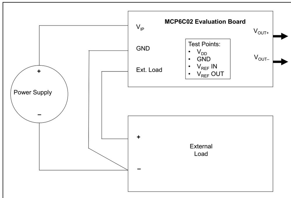
**FIGURE 1-1:** Using an External Load Block Diagram.
