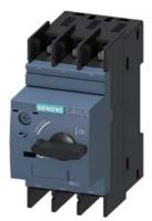
Circuit breaker size S0 for motor protection, CLASS 10 A-release 10...16 A N-release 208 A ring cable lug connection Standard switching capacity
