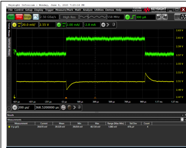
Figure 13. Load Transient, \pm 2 mA, V_{IN} = 5 V, C_{IN} = 1 \mu\text{F} , C_{OUT} = 1 \mu\text{F} , 20 mV/div
