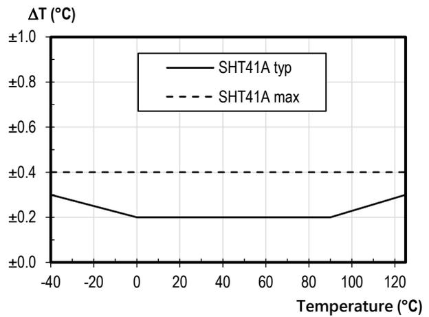
**Figure 7.** SHT41A typical and maximal temperature accuracy.
