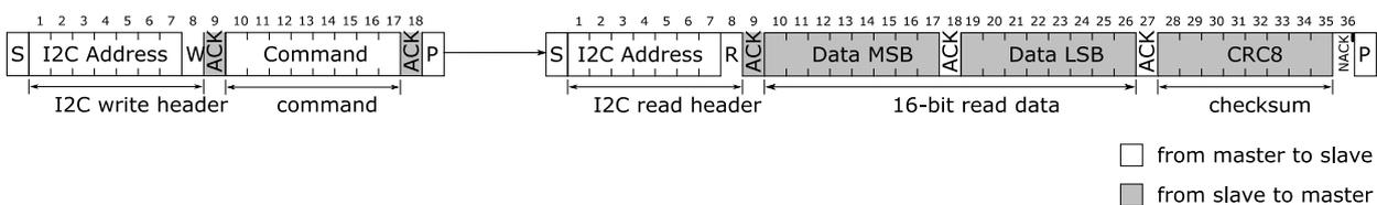
**Figure 8.** I2C transfer types: First a write header is sent to the I2C slave, followed by a command, for example “measure RH&T with highest precision”. After the measurement is finished the read request directed to this I2C slave will be acknowledged and transmission of data will be started by the slave.
