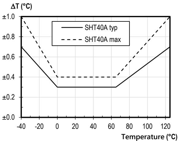
**Figure 6.** SHT40A typical and maximal temperature accuracy.
