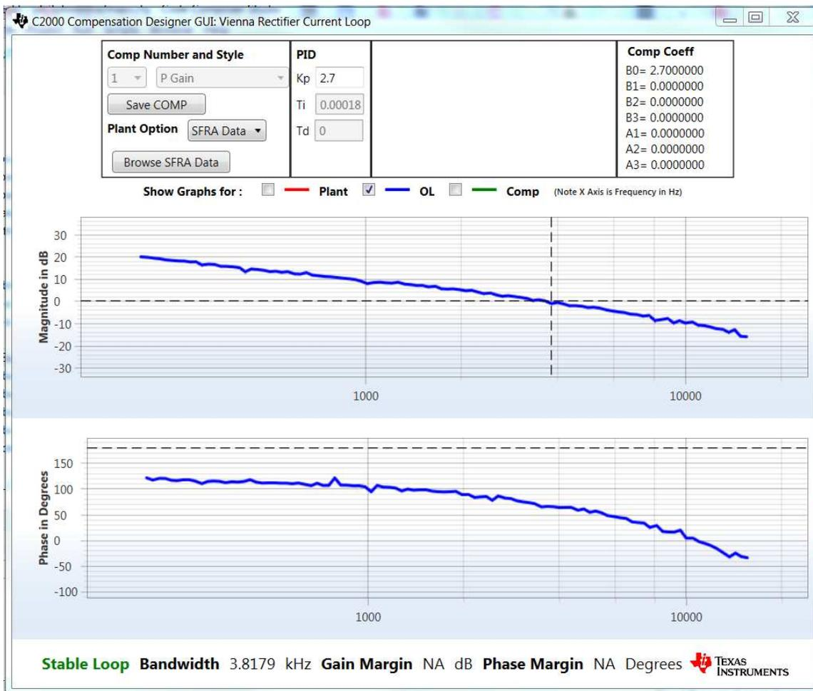
16. This action verifies the current compensator design. Note the phase is off because there is a negative sign in the control loop.
