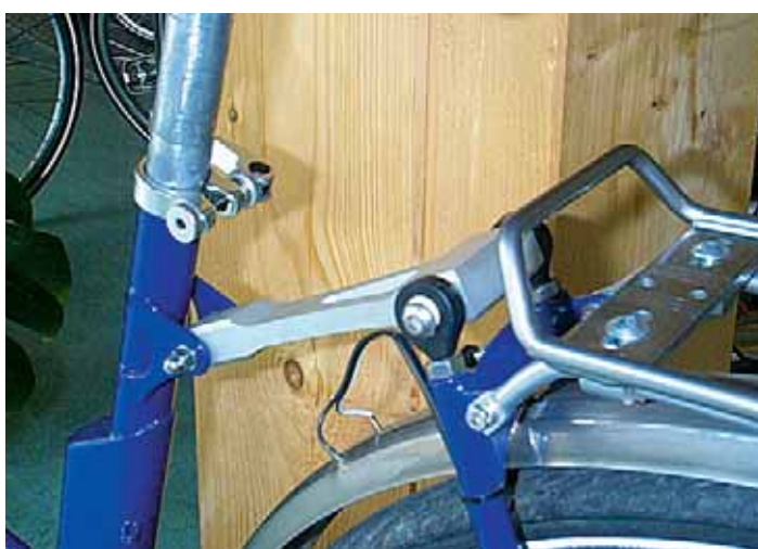
Picture 51.2: igubal® rod end bearings in the a bicycle rear suspension
