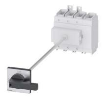
SENTRON, Switch disconnector 3LD, main switch, 4-pole, lu=250 A, Operating power / at AC-23 A at 400 V: 132 kW, floor mounting with door coupling, knob-operated mechanism, black, 4-hole mounting of the handle
