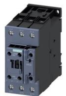
power contactor, AC-3e/AC-3, 65 A, 30 kW / 400 V, 3-pole, 20-33 V AC/DC, 50/60 Hz, with integrated varistor, auxiliary contacts: 1 NO + 1 NC, screw terminal, size: S2, upright mounting position
