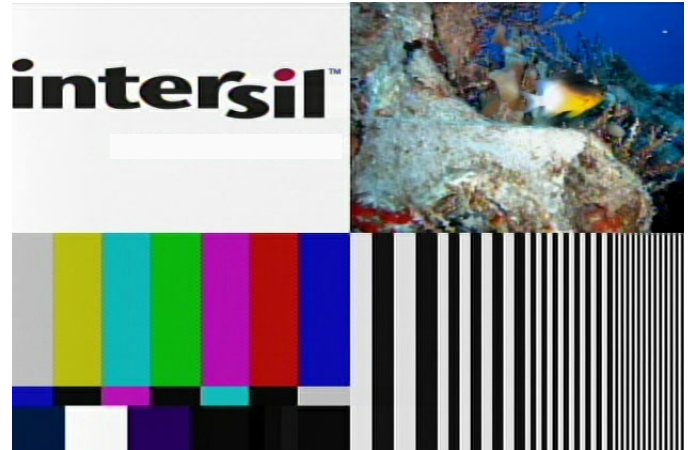
FIGURE 6. TEST PATTERN IMAGE AFTER 2000 FEET OF CAT 5 WITH ISL59602 (OR BETTER)
