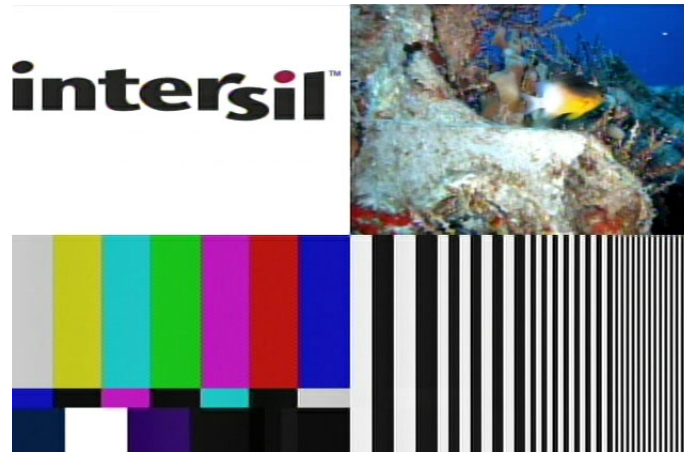
FIGURE 14. TEST PATTERN IMAGE AFTER 4000 FEET OF CAT 5 WITH ISL59604 (OR BETTER)
