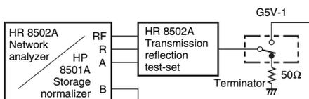
Terminals which were not being measured were terminated with 50  $\Omega$ .
