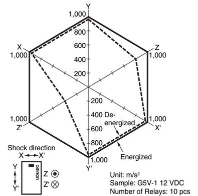
Test conditions: Shock is applied in  $\pm X$ ,  $\pm Y$ , and  $\pm Z$  directions three times each with and without energizing the Relays to check the number of contact malfunctions.
