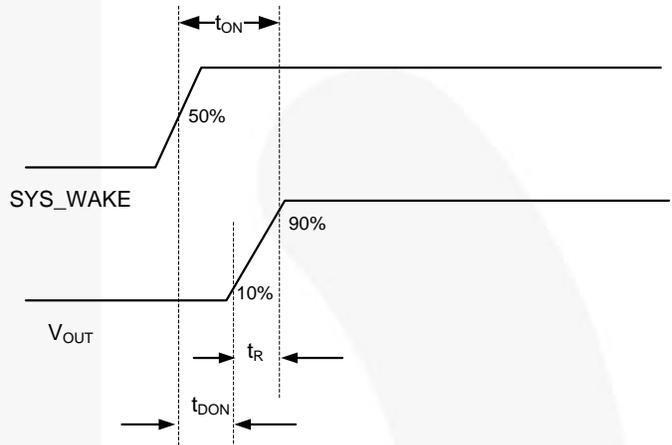
**Figure 29. Timing Diagram (SYS\_WAKE vs. V<sub>OUT</sub>)**
