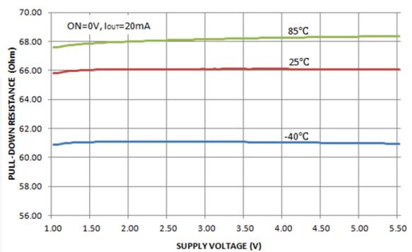
Figure 15. Output Discharge Resistor  $R_{PD}$  vs. Supply Voltage
