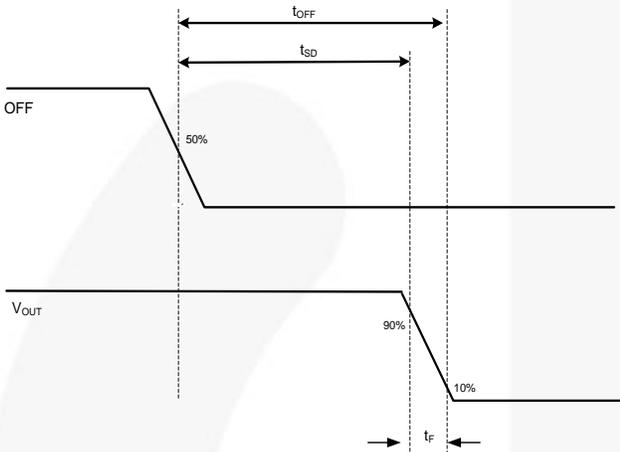
**Figure 28. Timing Diagram (OFF vs. V<sub>OUT</sub>)**
