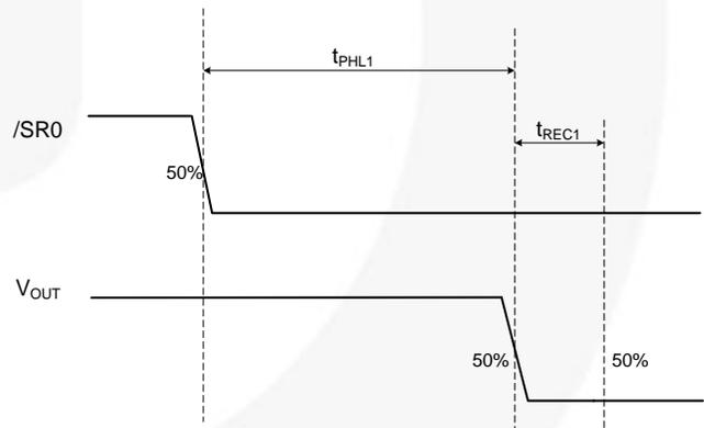
**Figure 31. Reset Timing**
