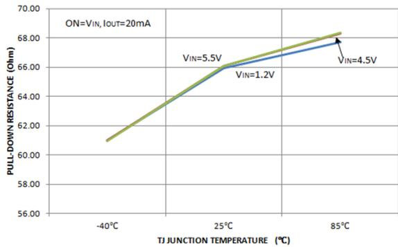
Figure 14. Output Discharge Resistor  $R_{PD}$  vs. Temperature
