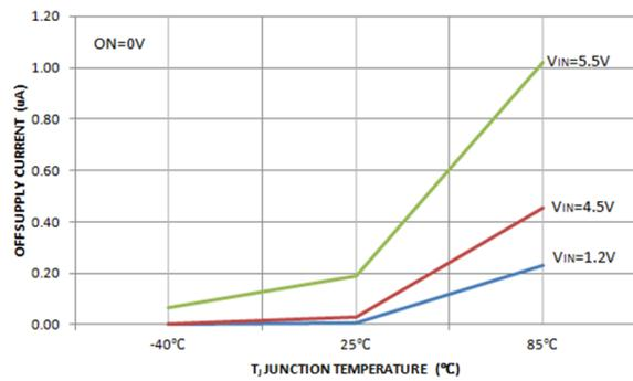
Figure 8. Off Supply Current vs. Temperature ( $V_{OUT}=0\text{ V}$ )
