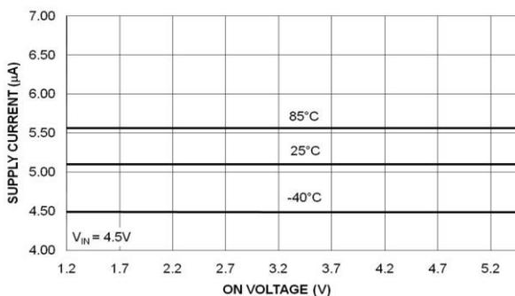
Figure 12. Quiescent Current vs. On Voltage ( $V_{BAT}=4.5\text{ V}$ )
