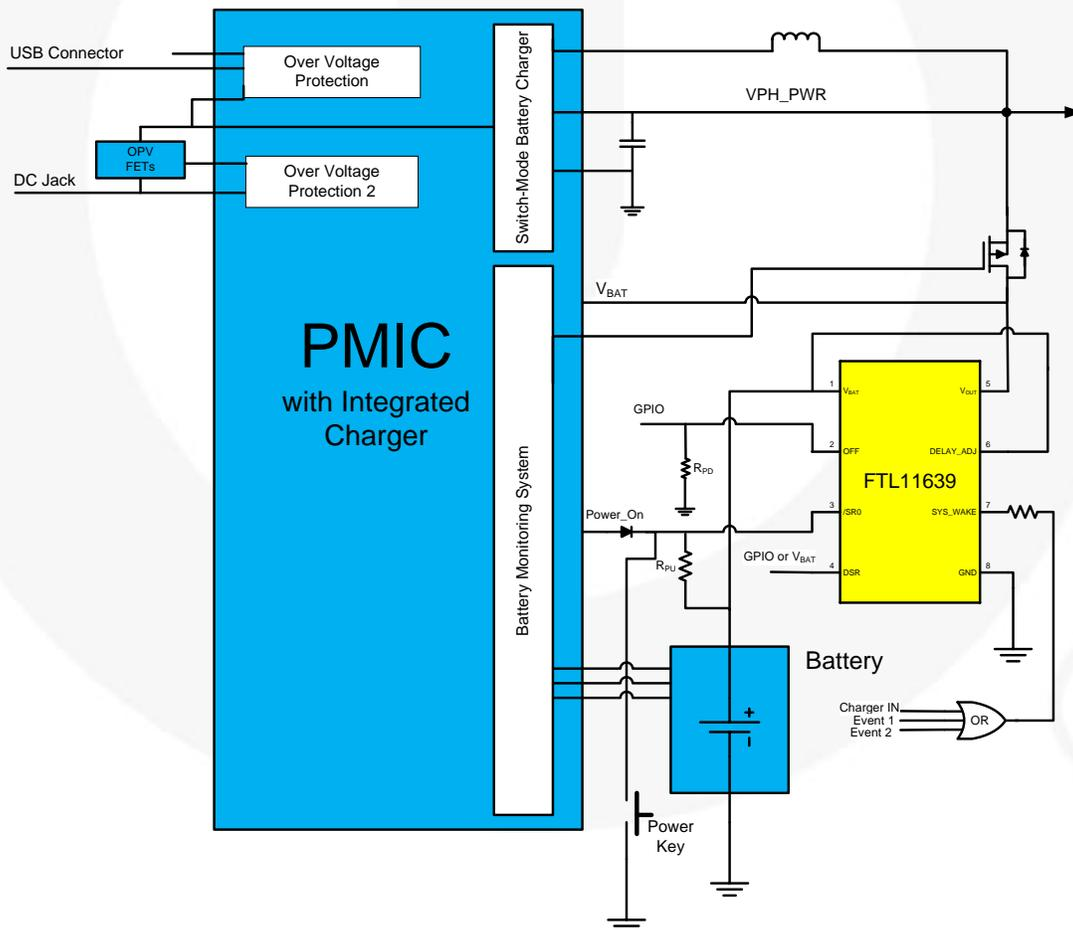
Figure 2. Typical Application PMIC with Integrated Charger
