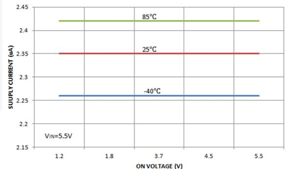
Figure 13. Quiescent Current vs. On Voltage ( $V_{BAT}=5.5\text{ V}$ )
