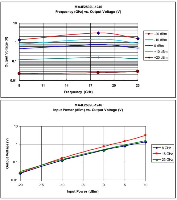
The MA4E2502L-1246 chip was evaluated in a detector circuit in which the Schottky diode terminates a 50 ohm transmission line on a duroid substrate. The chip was attached to the terminal of a 3.5mm connector and the output voltage was measured through a bias tee on a voltmeter. Matching was not attempted.
