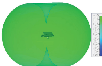
3D Gain Plot Side (700MHz)
