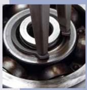
**Heavy duty tips:** optimum stability when loosening tight circlips
