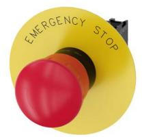
EMERGENCY STOP mushroom pushbutton, 22 mm, round, plastic, red, 40 mm, positive latching, acc. to EN ISO 13850, rotate-to-unlatch, with yellow backing plate, inscription: EMERGENCY STOP, with holder, 1 NC, screw terminal
