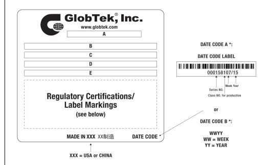
A=Medical/ITE/Household use Power Supply B=P/N: (料号) WR9QE500T00NAIMR6B C=Model (型号) GTM96060-0612 D=Input (输入) 100-240V~, 50-60 Hz, 0.6 A
