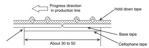
No lifting for the direction of progressing
