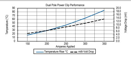
The graph shows the Dual Pole Power Clip electrical performance in terms of temperature rise and voltage drop at currents from 150A to 350A. The set up for the test consisted of the following:
