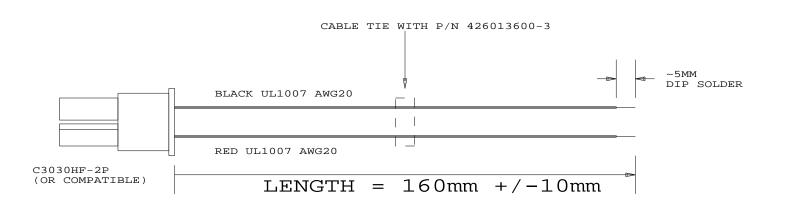
P/N 426013600-3 3MM POWER-IN CABLE 2WAY, 160MM DIGITAL VIEW LTD.
