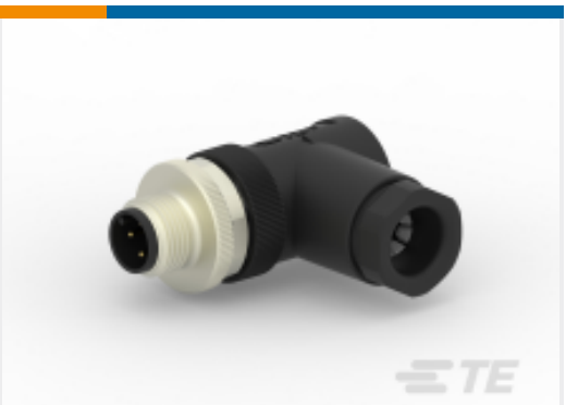
TE Part #T4113002041-000 M12,MALE,RA,A CODE,4P,PG9,GOLD
