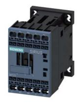
Power contactor, AC-3 9 A, 4 kW / 400 V 2 NO + 2 NC 220 V DC, 50 Hz/240 V, 60 Hz 4-pole Size S00 Spring-type terminals
