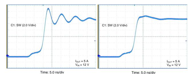
Figure 15. SW Voltage Without Snubber
