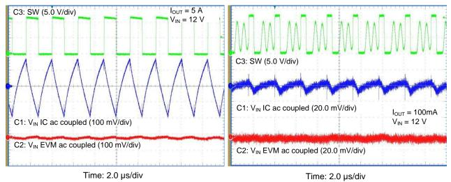
Figure 10. Input Voltage Ripple CCM
