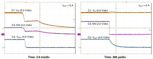
Figure 20. Shutdown Relative to VIN
