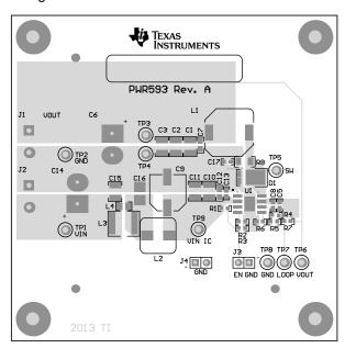
Figure 24. TPS54540-Q1EVM-593 Top Assembly and Silkscreen
