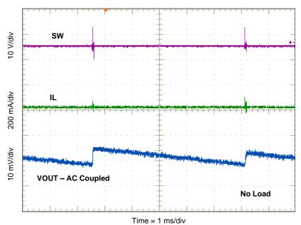
Figure 14. Output Voltage Ripple Eco-mode
