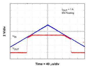
Figure 23. Low Dropout Start Up and Shutdown
