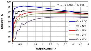
Figure 3. Efficiency versus Load Current
