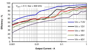
Figure 4. Light-Load Efficiency
