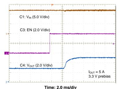
Figure 19. Prebias Start Up Using EN
