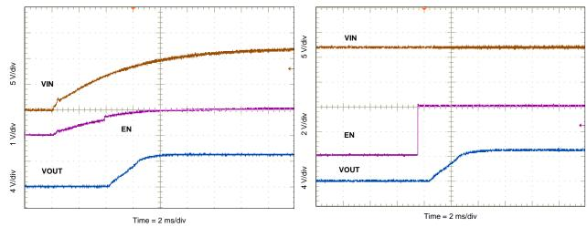
Figure 17. Start Up Relative to V<sub>IN</sub> Ramping Up
