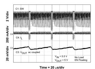
Figure 22. Low Dropout Operation
