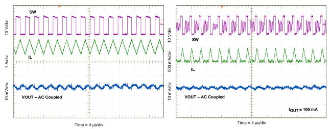
Figure 12. Output Voltage Ripple CCM
