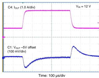
Figure 7. Load Transient Response
