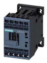
Power contactor, AC-3 9 A, 4 kW / 400 V 110 V AC, 50 Hz, 120 V, 60 Hz, 3-pole, Size S00 Spring-type terminal
