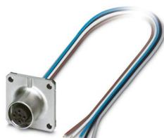
Device connector front mounting, 5-position, Socket, straight, M12, coding: B, on free cable end, Front mounting, Square flange, Individual wires, cable length: 0.5 m, 0.34 mm<sup>2</sup>, TPE litz wire
