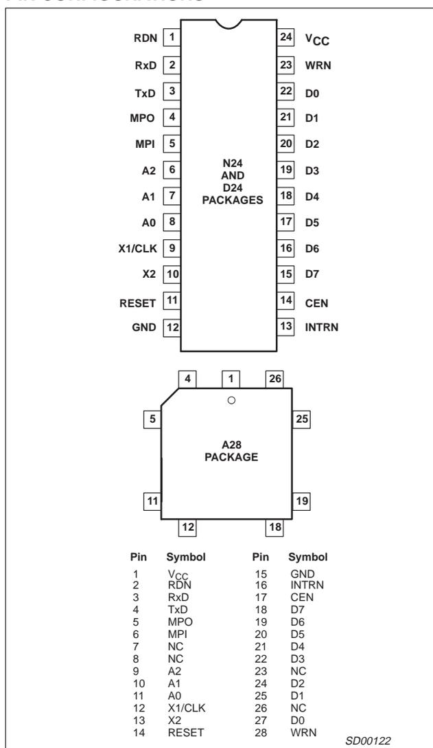
Figure 1. Pin Configurations
