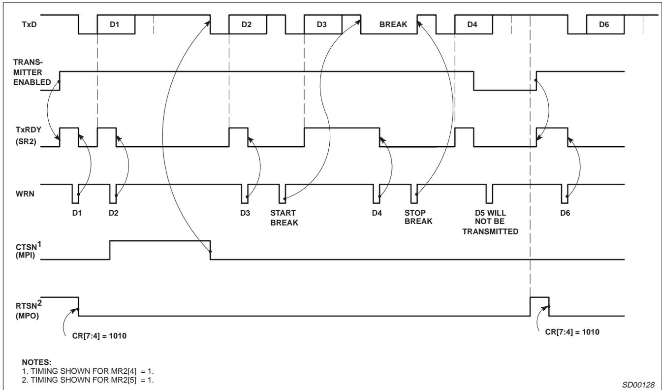
Figure 10. Transmitter Timing
