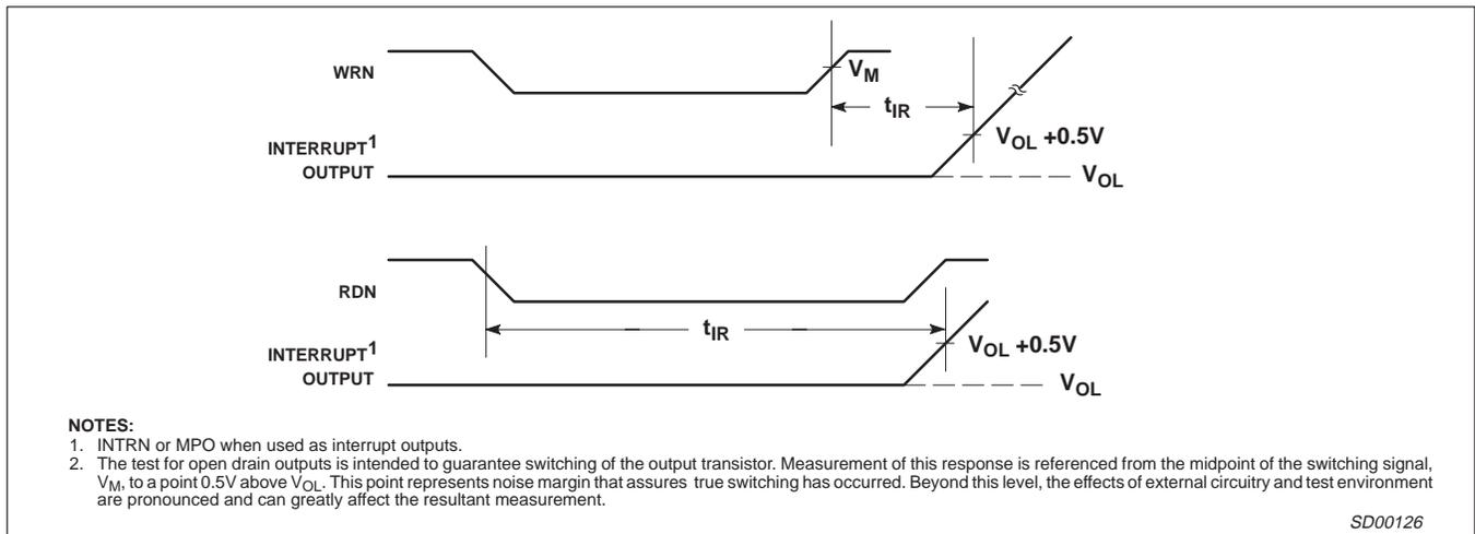
Figure 6. Interrupt Timing
