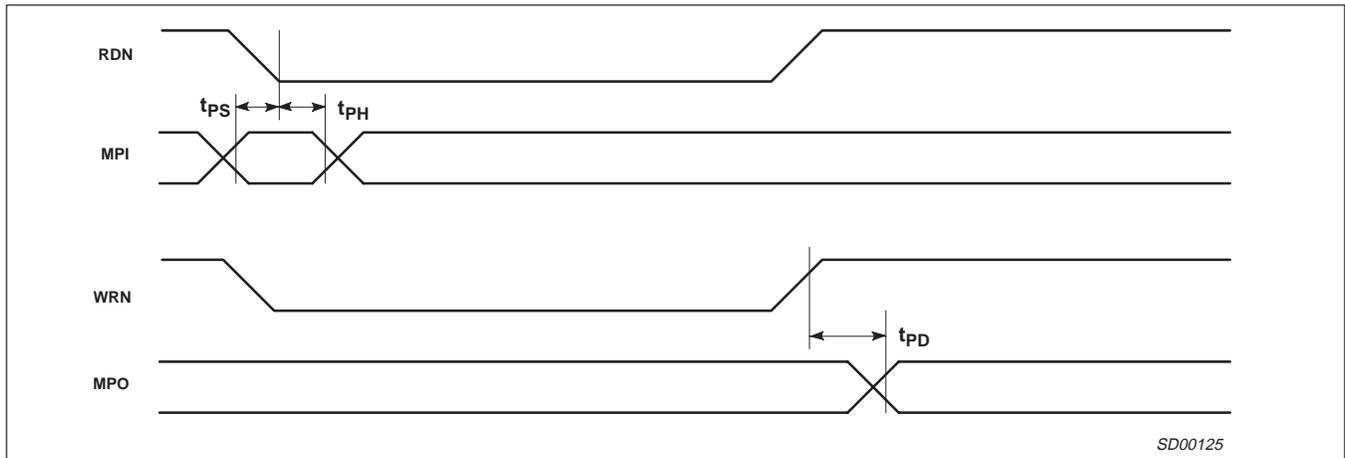
Figure 5. I/O Timing
