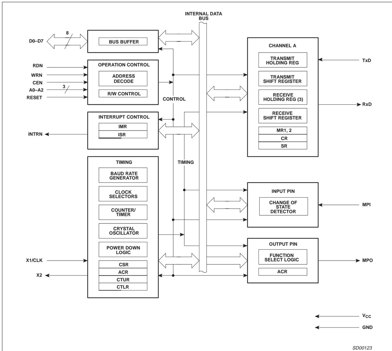
Figure 2. Block Diagram
