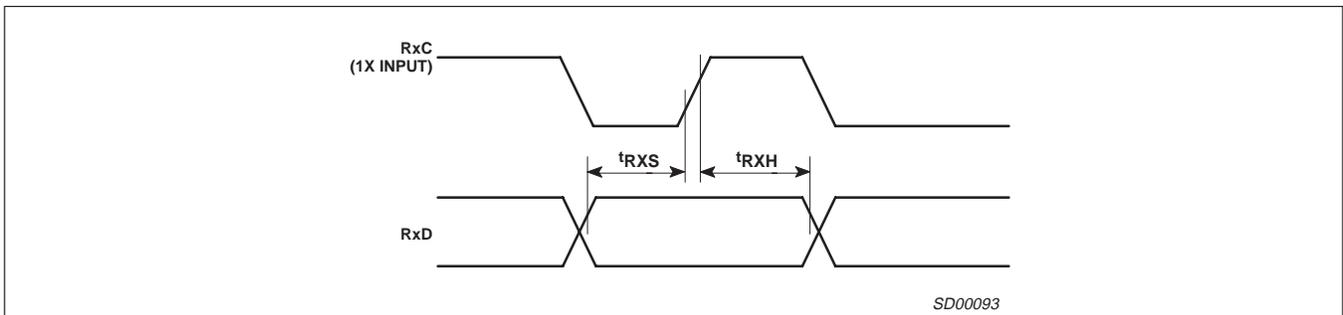
Figure 9. Receive Timing
