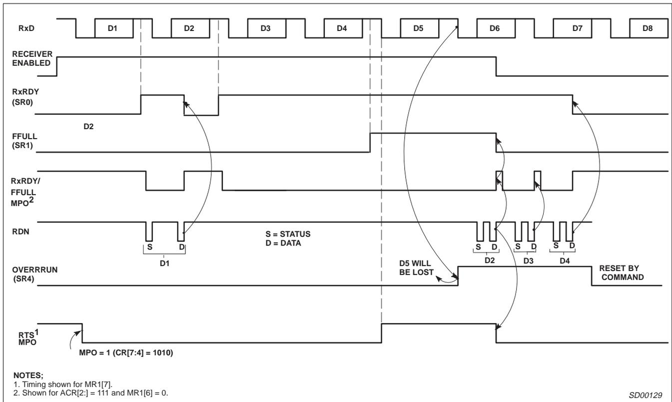
Figure 11. Receiver Timing
