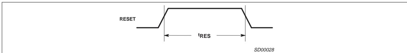
Figure 3. Reset Timing
