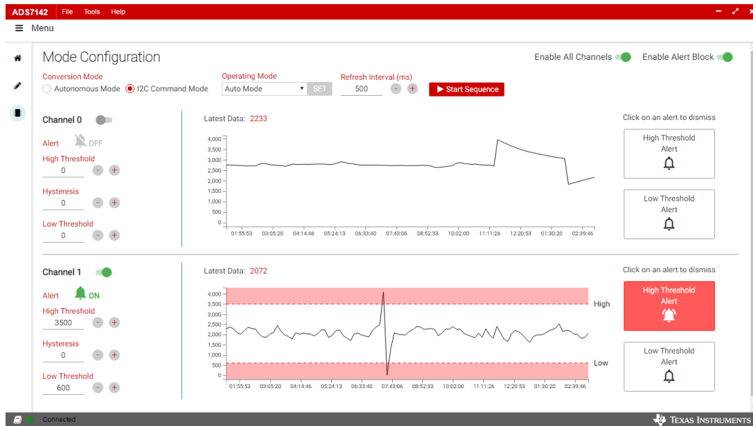
Figure 121. Alert Output from ADS7142 with PIR Sensor
