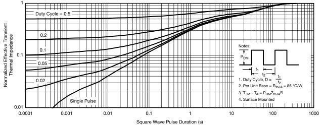
Normalized Thermal Transient Impedance, Junction-to-Ambient
