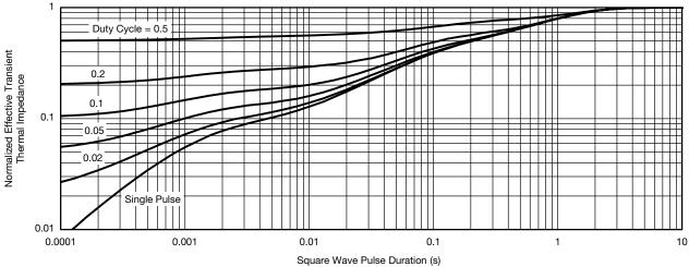
Normalized Thermal Transient Impedance, Junction-to-Foot
