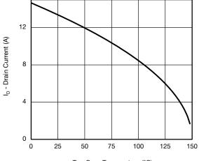
T<sub>C</sub> - Case Temperature (°C) **Current Derating\***
