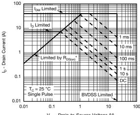
$V_{DS}$  - Drain-to-Source Voltage (V) \*  $V_{GS}$  > minimum  $V_{GS}$  at which  $R_{DS(on)}$  is specified
