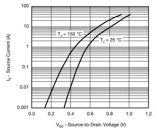
Source-Drain Diode Forward Voltage
