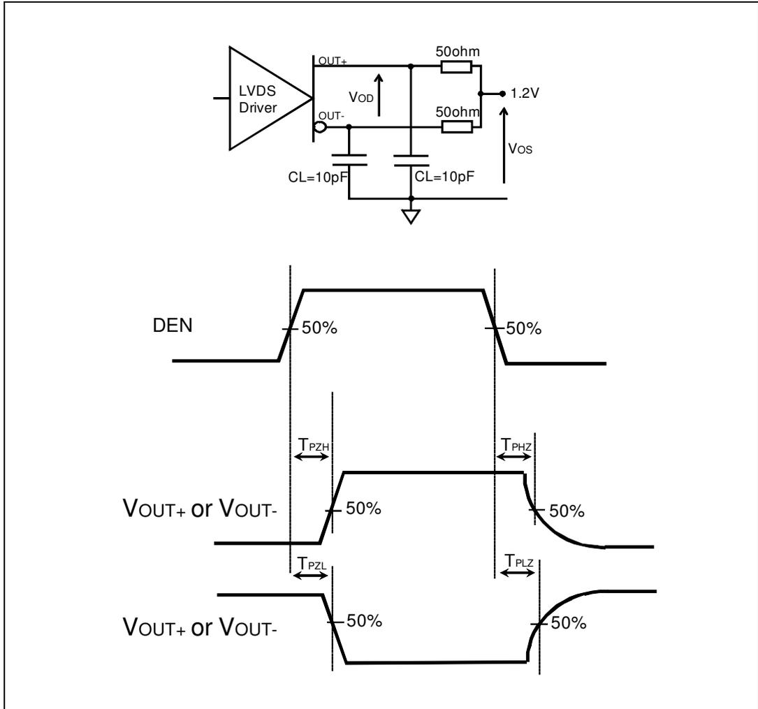
1. All input pulses are supplied by a generator with the following characteristics:  $t_r$  or  $t_f \leq 1$  ns,  $f_{REN}$  or  $f_{DEN} = 500$  kHz, and pulse width  $REN$  or  $DEN = 500$  ns.
