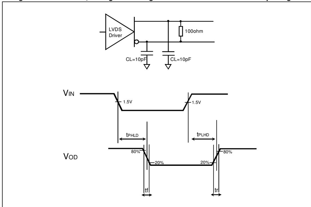
1. All input pulses are supplied by a generator with the following characteristics:  $t_r$  or  $t_f \leq 1$  ns,  $f = 1$  MHz,  $Z_O = 50 \Omega$ , and duty cycle = 50%.
