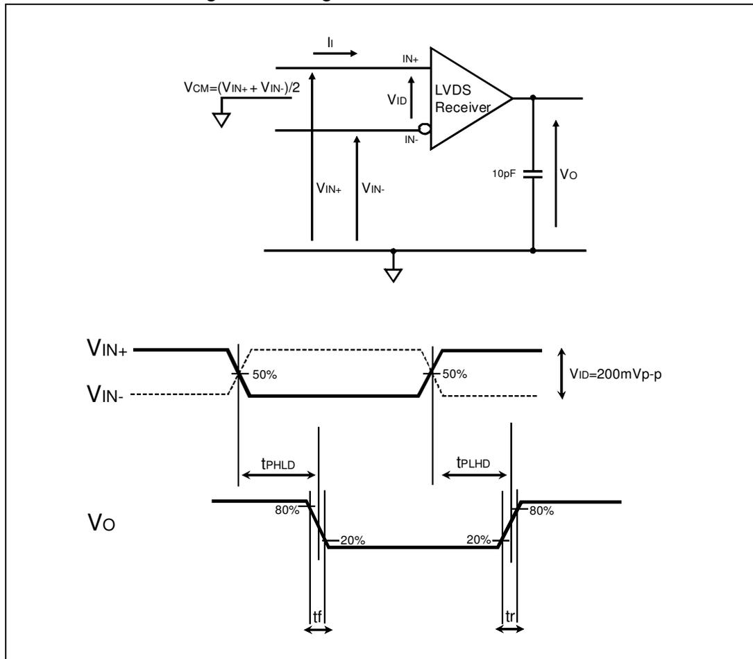
1. All input pulses are supplied by a generator with the following characteristics:  $t_r$  or  $t_f \leq 1$  ns,  $f = 1$  MHz,  $Z_O = 50 \Omega$ , and duty cycle = 50%.
