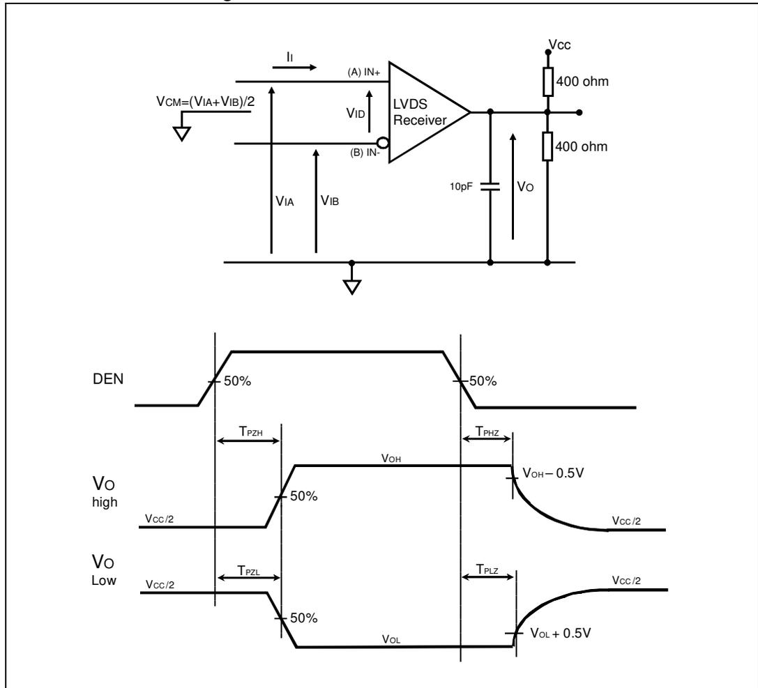
1. All input pulses are supplied by a generator with the following characteristics:  $t_r$  or  $t_f \leq 1$  ns,  $f_G$  or  $f_{\bar{G}} = 500$  kHz, and pulse width  $G$  or  $\bar{G} = 500$  ns.
