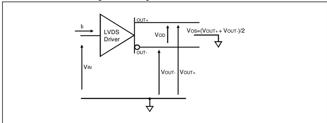
Figure 3. Test circuit, timing and voltage definitions for differential output signal
